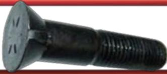
This plow bolt features a flat, round, countersunk head with a single reverse key that prevents the head from turning. Also, when replacing bolts, the key insures that the bolt is placed in its original position. No. 7 Bucket Tooth Plow Bolts are often used on heavy equipment such as snow plows and road graders. Parts meet SAE J429 Grade 8 specifications.
