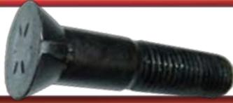
Coarse Thread. This plow bolt features a flat, round, countersunk head with a single reverse key that prevents the head from turning. Also, when replacing bolts, the key insures that the bolt is placed in its original position. No. 7 Bucket Tooth Plow Bolts are often used on heavy equipment such as snow plows and road graders. Parts meet SAE J429 Grade 8 specifications.
